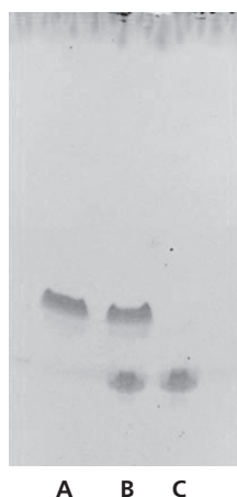
Figure 3 TLC analysis of the PEG-lipid (A), the mixture (B) of PEG-lipid and mPEG-amine, and mPEG-amine (C)
